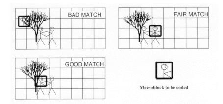
**Motion Estimation Macroblock:** Predicted candidate Frame 2 can be generated from Frame 1 by subtracting it from the desired frame, leaving a (hopefully) less complicated residual error frame that can then be encoded much more efficiently than before motion estimation.
