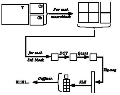
The basic processing blocks shown are the video filter, discrete cosine transform, DCT coefficient quantizer, and run-length amplitude/variable length coder. These blocks are described individually in the sections below or have already been described in JPEG Compression.
