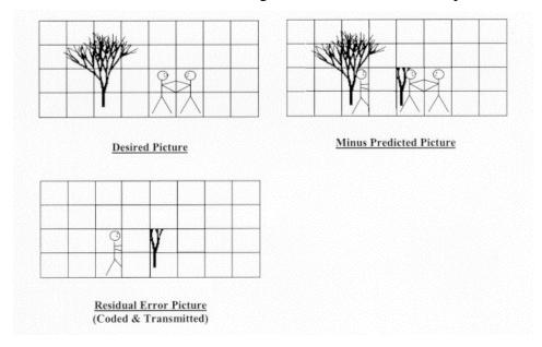
**Final Motion Estimation Prediction:** Not every macroblock search will result in an acceptable match. If the encoder decides that no acceptable match exists (again, the "acceptable" criterion is not MPEG defined, and is up to the system designer) then it has the option of coding that particular macroblock as an intra macroblock, even though it may be in a P or B frame. In this manner, high quality video is maintained at a slight cost to coding efficiency.
