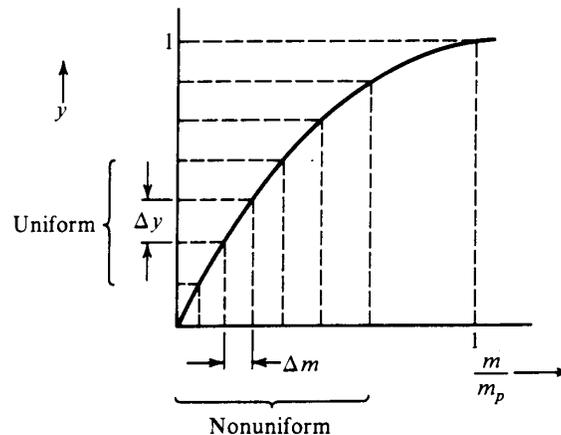
Figure 6.25 A Compandor for mapping non-uniform input levels to uniform ones.
