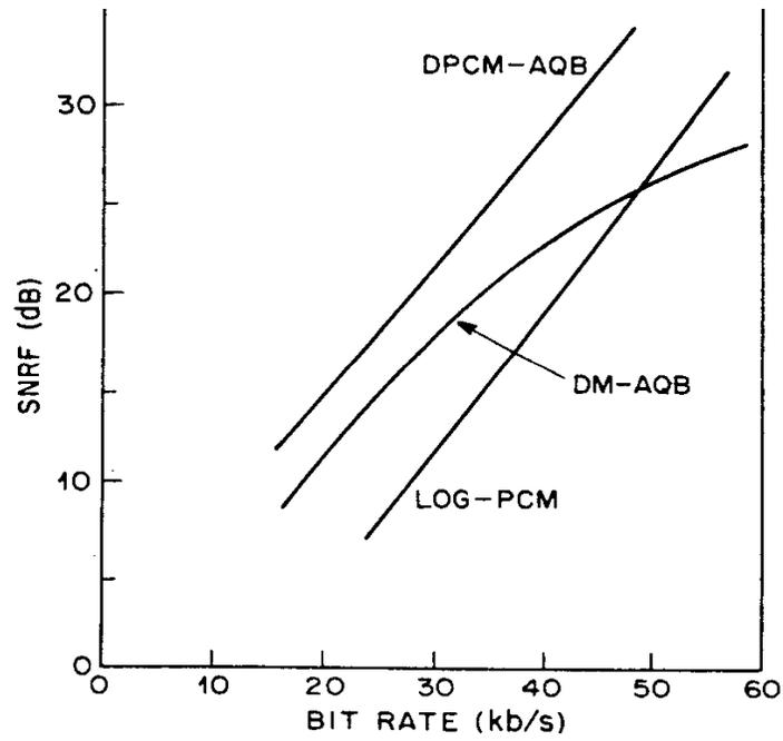
Figure 6.34 Comparative performance curves for PCM, DPCM and DM systems. (Reprint from Modern Analog and Digital Communication Systems, Third Edition, B. Lathi, courtesy of Oxford Press)
