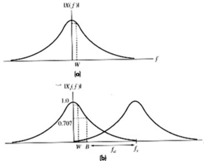
Figure 6.9 (a) Output of an RC filter used as a reconstruction filter; (b) After sampling. The segment between the origin and the frequency  $B$  represents the aliasing spillover the passband.
