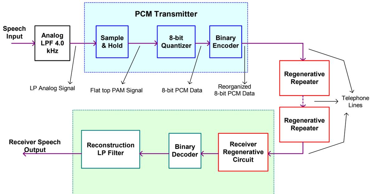
Figure 6.16 End-to-end single channel PCM block diagram.
