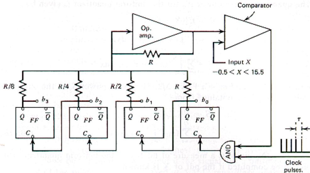
Figure 6.20 4-Bit (16-level) uniform quantizer circuit using discrete components.
