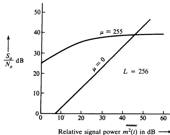
Figure 6.26 Performance of a companded and uniform quantizers.
