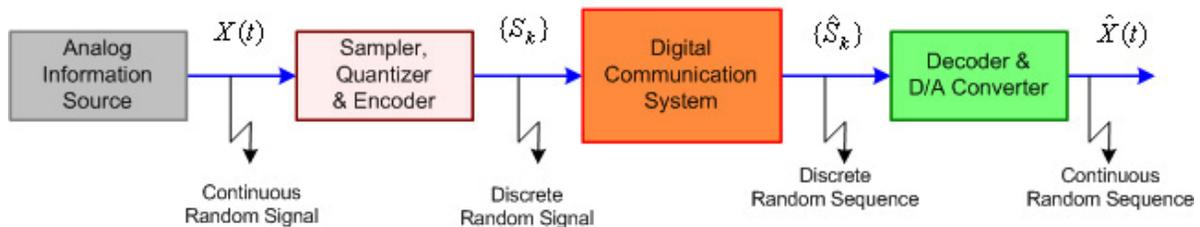
Figure 6.1 Transmission of analog signals using digital communication systems.
