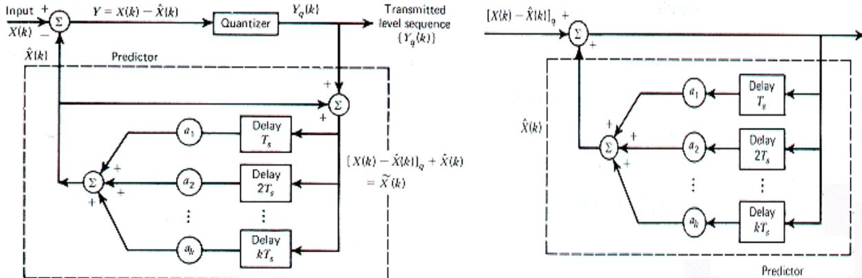
Figure 6.28 Differential Quantizing Techniques. Transmitter and receiver Circuits.
