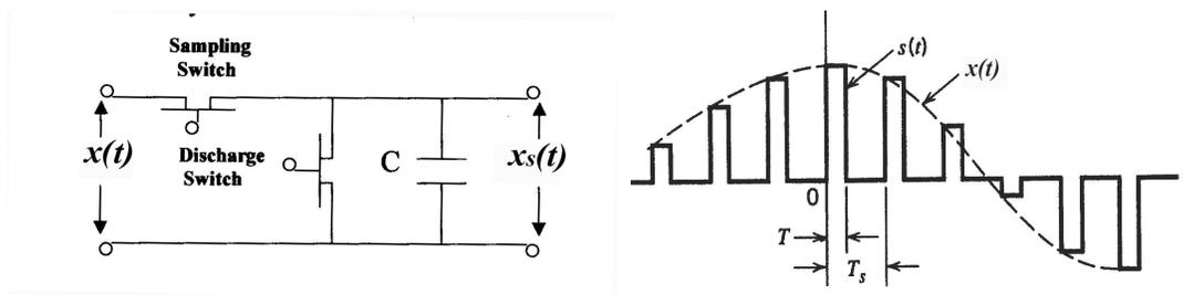
Figure 6.11 Practical flat-top PAM sampling using two-transistor switches.
