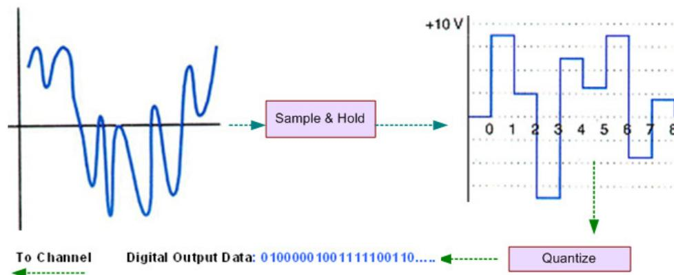
Figure 6.2. Sampling and quantization of analog signals.
