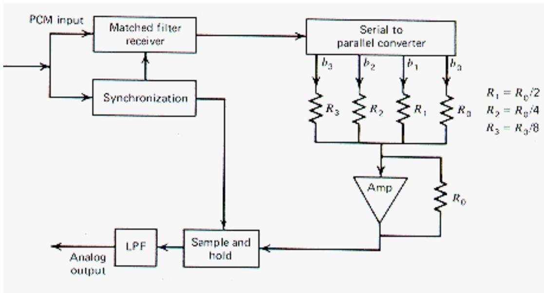
Figure 6.22 Components of a PCM Receiver for a PCM System with Uniform Quantizer.
