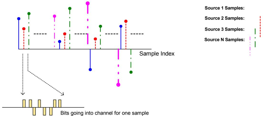
Figure 6.13b Fusion of quantized data from N sources into a TDM data string using Commutator.
