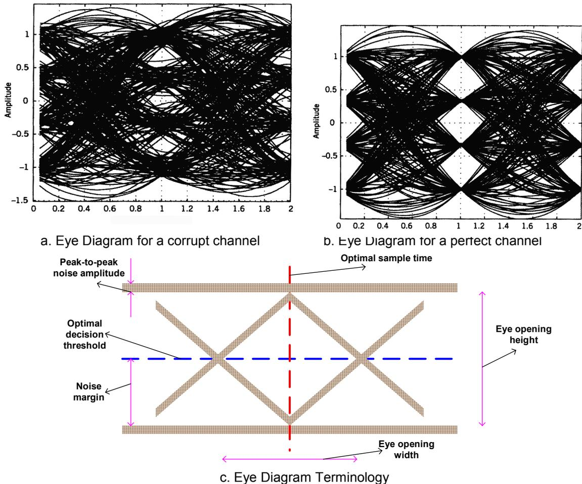
Figure 6.17 Open and closed eye diagrams and the terminology
