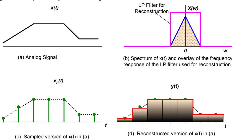
Figure 6.6 Reconstruction of the analog signal with an ideal LP filter.
