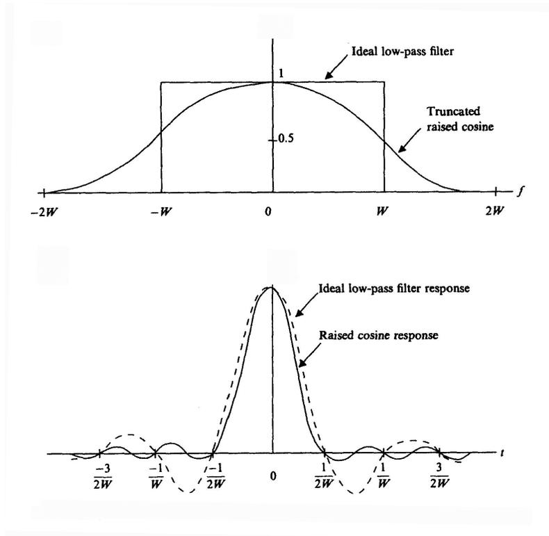
Figure 6.18 Frequency and impulse responses of a raised cosine pulse.
