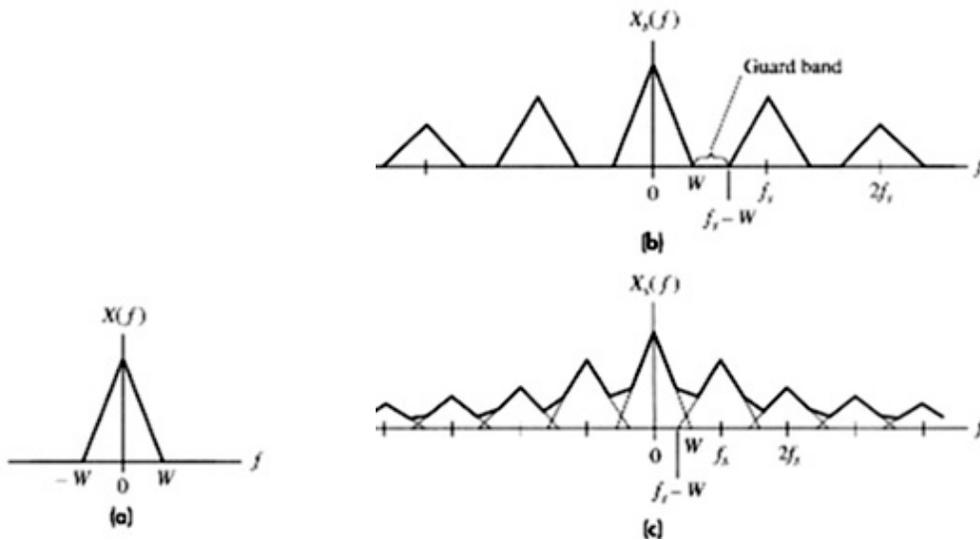
Figure 6.5 (a) Spectra for the baseband signal. (b) Spectrum of the sampled signal when  $f_S > 2W$  and (c) Spectrum of the sampled signal when  $f_S < 2W$  resulting in spectral fold-over.
