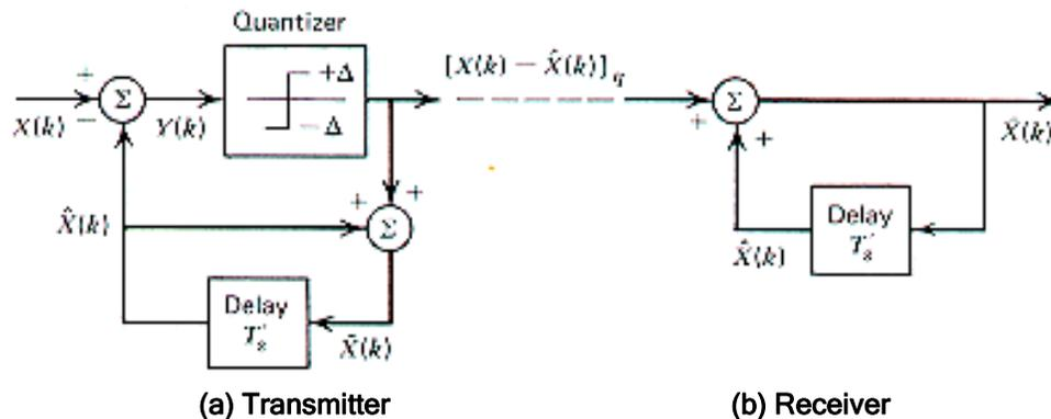
Figure 6.29 Functional block diagram of a linear DM system.
