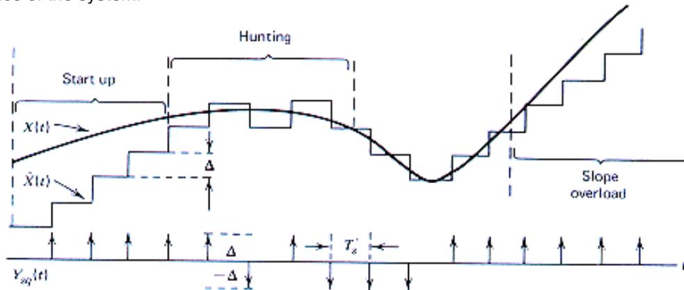
Figure 6.31 Delta Modulation signal and its staircase approximation.
