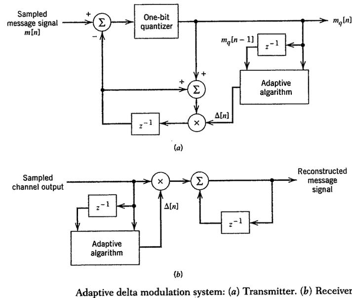
Figure 6.33. Transmitter and receiver blocks for the adaptive DM system in Example 6.9.
