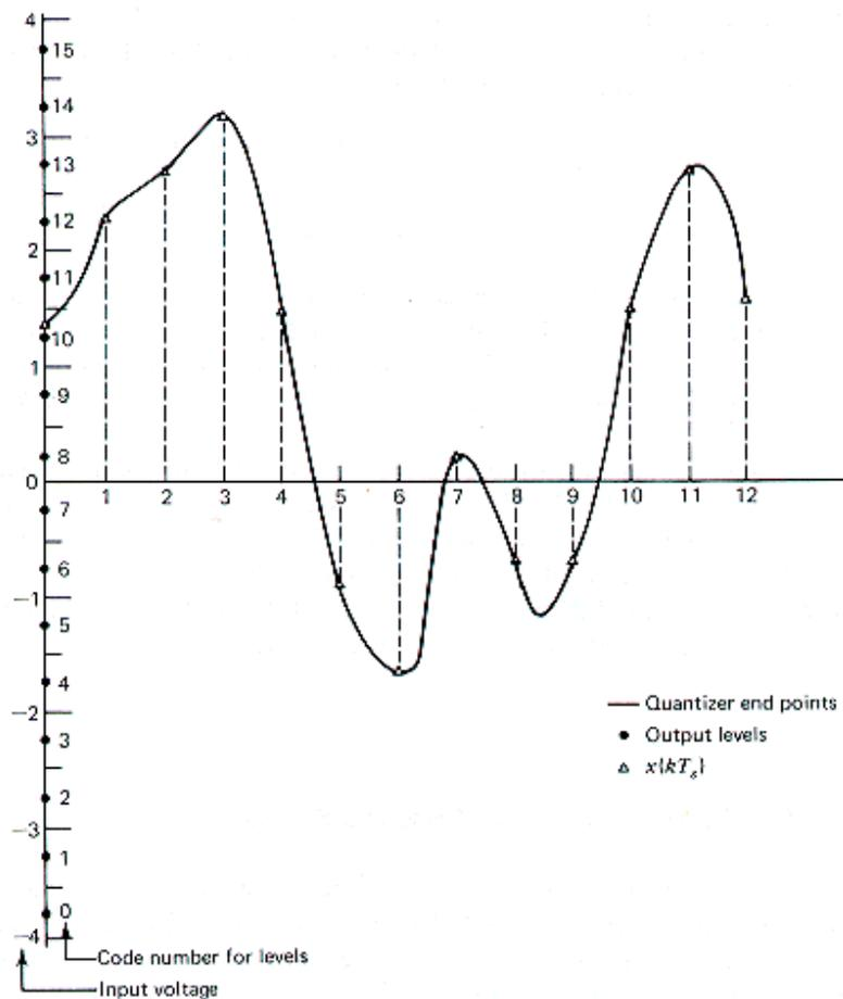
Figure 6.21 Quantization of an analog signal  $x(t)$  with the 4-bit uniform quantizer of Figure 6.20.
