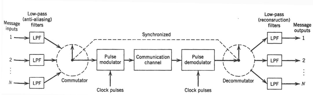
Figure 6.13a Illustration of Time-Division Multiplexing (TDM).
