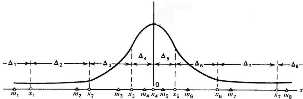
Figure 6.24 Illustration of a 3-bit non-uniform quantization.
