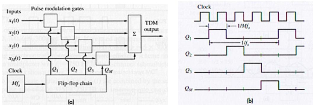
Figure 6.14 TDM Commutator (a) and timing diagram (b).
