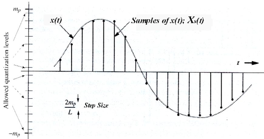
Figure 6.23 PCM using an  $M$ -level uniform quantizer.
