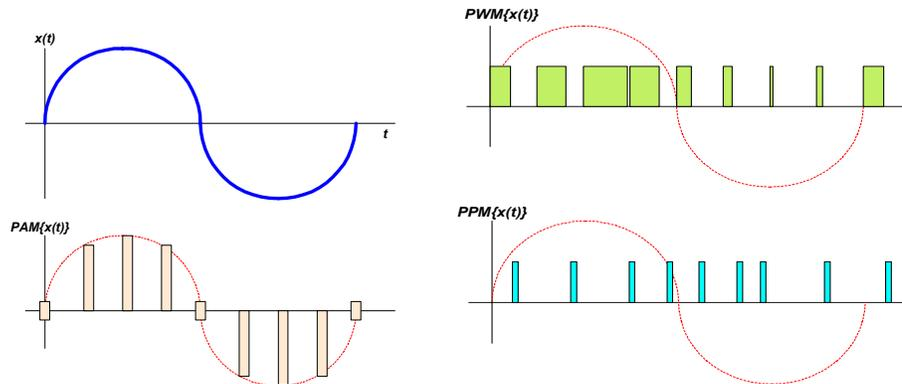
Figure 6.12 PAM, PWM and PPM sampling of analog signals.
