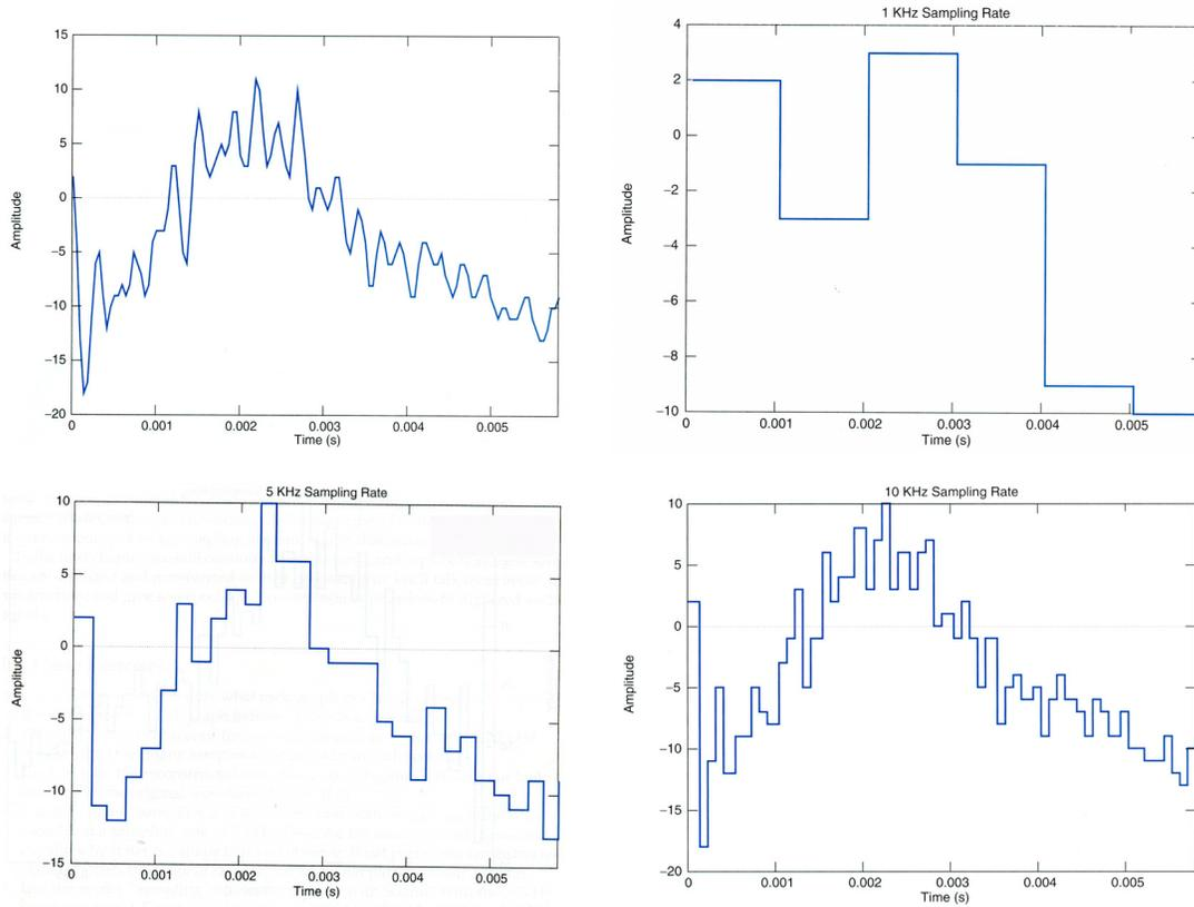
Figure 6.3 Effect of sampling rate on speech signals.
