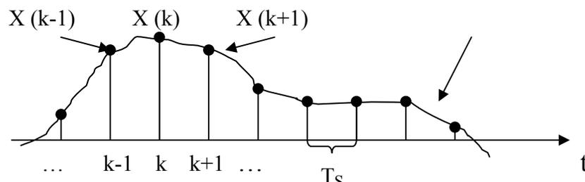
Figure 6.27 A continuous signal and its samples to explain the differential coding schemes.
