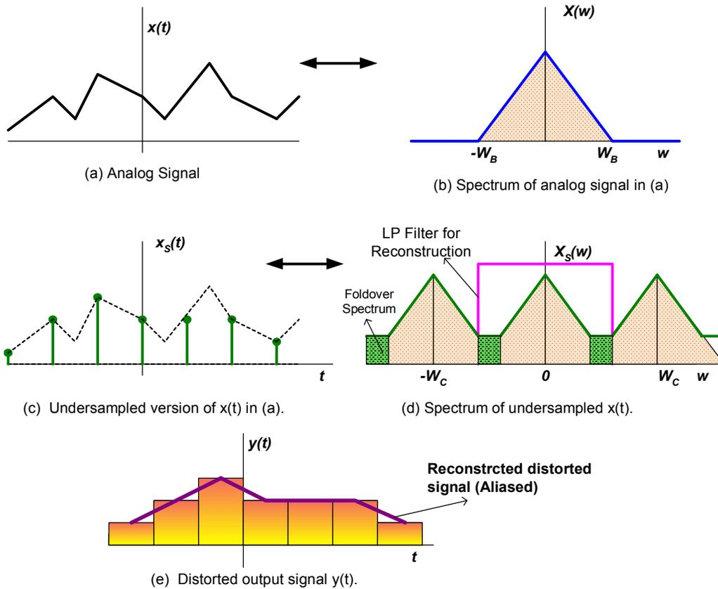
Figure 6.10. Effects of under-sampling (aliased) on reconstructed signal.
